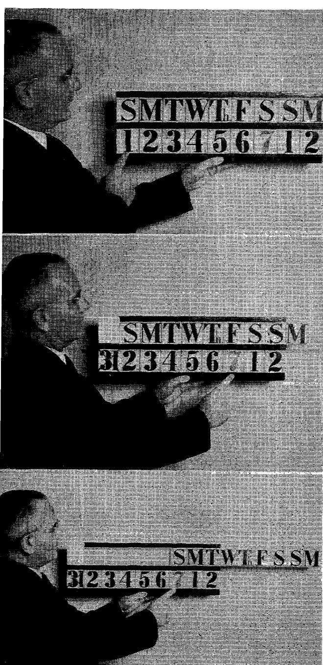
FIGURE 1: Calendar device in starting position, showing seven-day weekly cycle in figures on the bottom row, with the days of the week above.
